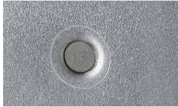
RESULT OF THE INSTALLATION OF SELF-PIERCING RIVET
