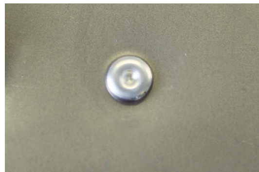
RESULT OF THE INSTALLATION OF A FLOW-FORM RIVET
