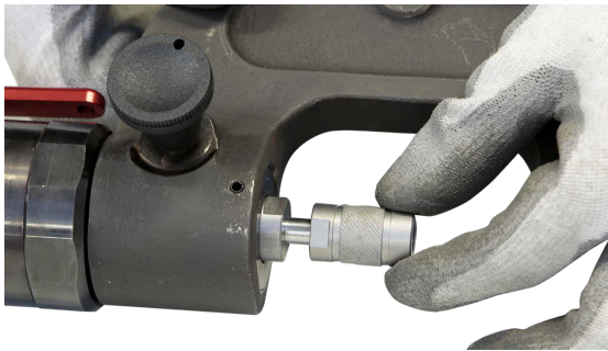
Using the screw, fasten the extension supplied with the arm.
